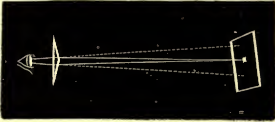
FIG. 163.—Action of the double prism.
